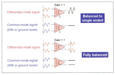
▲ Figure 1. Two types of differential components, with singleended and a differential output.
