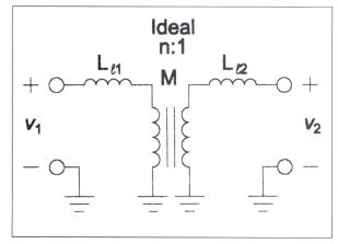
▲ Figure 2. Lossless transformer model.
