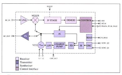
▲ Figure 1. Block diagram of the CC1000.
