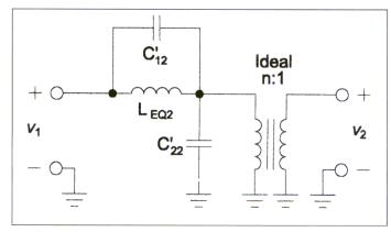
ightharpoonup Figure 7. Equivalent circuit for determining  $oldsymbol{\mathcal{C}'}_{11}$ .
