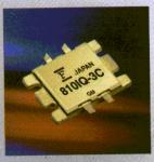
FLL8101Q-3C f=2.6 GHz Pout=49.0 dBm (Typ.) GL=12.0 dB (Typ.)
