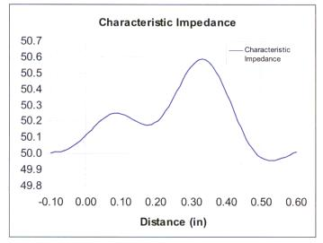
▲ Figure 3. TDR for the glass bead text fixture of Figure 2 and Table 1.
