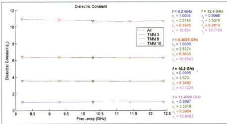
▲ Figure 4. Measurement results of air: TMM 3, TMM 6 and TMM 10.
