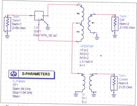
Figure 8. A circuit simulator may also be used to measure mixed-mode parameters of the differential device.
