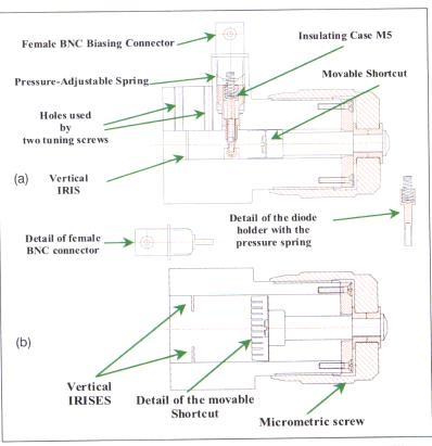
Figure 1. Mechanical drawing of the waveguide Gunn oscillator, showing (a) transversal view and (b) top view.
