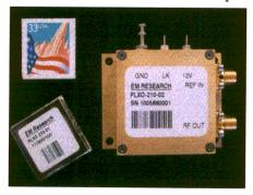
hertz phase noise at 10 kHz offset. Available in 1-inch square surfacemount or connectorized 1.5-inch square packages, the PLXO Series is ideally suited for use as high stability low phase noise reference (clock) oscillators.
