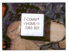
sideband phase noise of -82 and -107 dBc per hertz at 10 and 100 kHz, respectively. The device also delivers 4 ±2 dBm into a 50-watt load with nominal 4.25 volt supply while drawing less than 25 mA.
