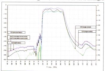
lacktriangle Figure 5. Offset between the values of  $S_{31}$  and  $S_{21}$  represents the overall balance between the two terminals that make up the differential port. This image also contains the comparison of the balun and mixed-mode methods.
