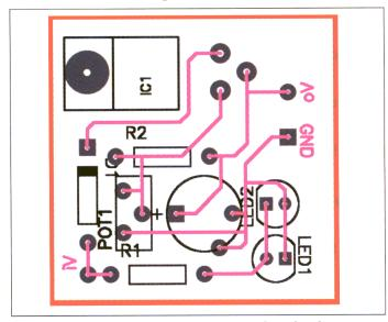
▲ Figure 4(b). PCB layout of the protection circuit.
