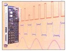
eration with major aircraft engine and power systems manufacturers to provide the features needed for accurate simulation of real-world sensor inputs. The V370 is ideal for simulation of sensor signals from complex rotating machines, generation of pure and distorted polyphase AC waveforms, generation of complex pulse trains with realtime control of relative pulse positions and amplitudes and shake table, servo or actuator drive.
