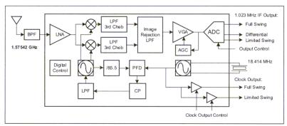
Figure 1. GPS front end block diagram.
