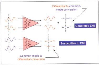
▲ Figure 2. Mode conversion occurs when some of the differential signal is converted into the common mode and some of the common-mode signal is converted into the differential mode.
