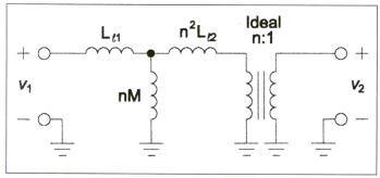
▲ Figure 3. Lossless transformer model referred to primary side
