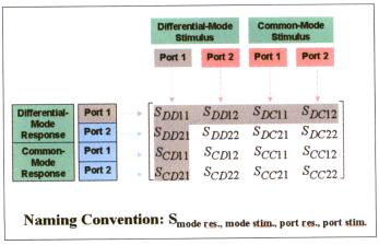
▲ Figure 3. A mixed-mode S-matrix can be organized in a similar way to the single-ended S-matrix, in which each column represents a different stimulus condition, and each row represents a different response condition.
