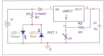
▲ Figure 4(a). Diagram of the protection circuit.
