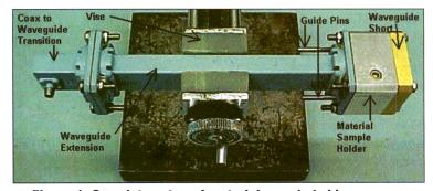
▲ Figure 1. Complete setup of material sample holder.
