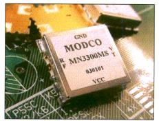
frequency. Offering up to 5 percent tuning bandwidths over a range of 2.4 to 4.2 GHz, the MN series operates on +5 VDC at less than 35 mA current. The MN series VCO is supplied in standard  $0.5 \times 0.5 \times 0.13$  inch surface-mount housing and is also available in UM series, offered in a  $0.35 \times 0.35 \times 0.10$  inch surface-mount package.
