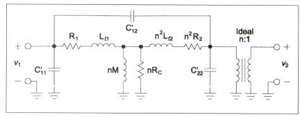
▲ Figure 8. Complete wideband transformer model.
