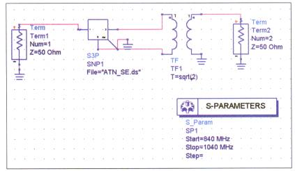
▲ Figure 7. The single-ended data is imported into Agilent's Advanced Design System (ADS) simulation tool, where it can be transformed to differential data using a balun circuit component.
