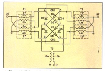
▲ Figure 1. Schematic of the mixer.
