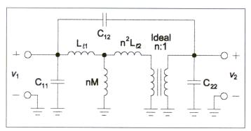
Figure 4. Wideband transformer model.
