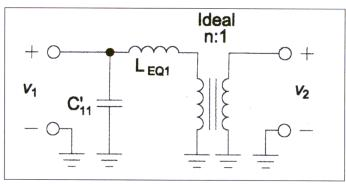
$\blacktriangle$  Figure 6. Equivalent circuit for determining  $C'_{12}$  and  $C'_{22}$ .
