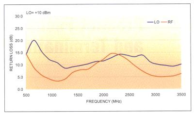
Figure 5. LO and RF return loss of the MCA-35LH.
