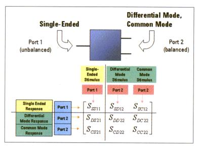
Figure 4. When the four-terminal matrix is converted to a threeterminal matrix, the differential and common modes on the differential ports and one mode on the single-ended port must be considered. The S-matrix for this configuration is arranged with the stimulus conditions in the columns and the response conditions in the rows.
