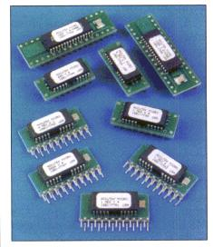
DRAM DIP and a 128 K  $\times$  8 SRAM DIP with 0.300 mil and 0.400 mil lead row centers.
