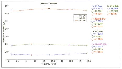
▲ Figure 3. Measurement results of MC 20, MC 25 and MC 50.
