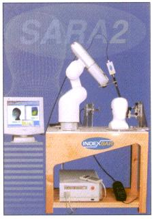
mm, the system can measure SAR from mobile telephones and other wireless devices using an upright generic phantom head.
