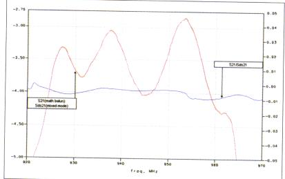
Figure 9. The error due to the mode conversion of the device can be calculated by comparing the mathematical balun results to the mixed-mode results.
