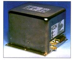
for radio-navigation applications. The RAFS exhibits short-term stability of less than 5  $\times$  10<sup>-14</sup> per 10,000 seconds and drift of less than 3  $\times$  10<sup>-13</sup> per day.
