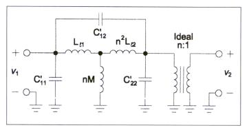
Figure 5. Wideband transformer model referred to primary side.
