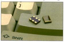
from ± 25 to 100 ppm, -40 to +85 degrees Celsius operation with tristate and tight (45/55 percent) symmetry. Low jitter and phase noise performance make the UVV ideal for SONET/SDH/ATM, optical carrier, DWDM, WDM, gigabit ethernet and fiber channel, PLL and clock recovery applications.
